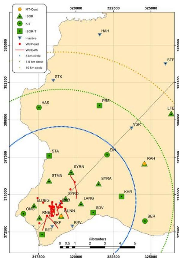
**Figure 1: Distribution of seismic monitoring stations and wells in the conventional geothermal field at the Reykjanes site (Iceland). A total of 19 seismic were deployed in a 10 km radius from the RN-15/IDDP-2 well.**
