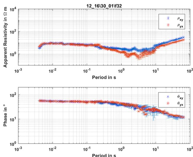
**Figure 1: Electric resistivity and phase versus period from the magnetotelluric monitoring from two monitoring days in December 2017 at station GUN. Blue curves show the XY-component, the red curves the YX-component.**
